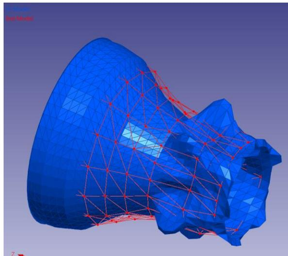
Figure 5 Correlation between measured and theoretical mode
