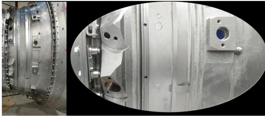
Figure 4 Geometrical features neglected in the model
