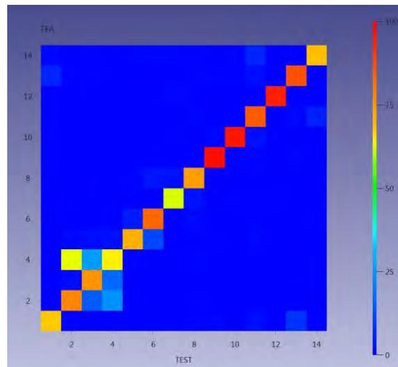
Figure 2 Correlation between the modal data obtained from vertical (Y-axis) and horizontal (X-axis) setup
