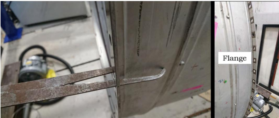
Figure 3 Measurement of the casing thickness
