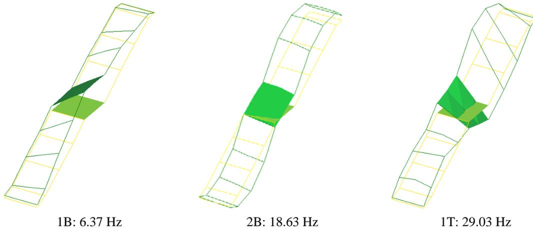
Figure 9. Mode shapes and natural frequencies obtained experimentally
