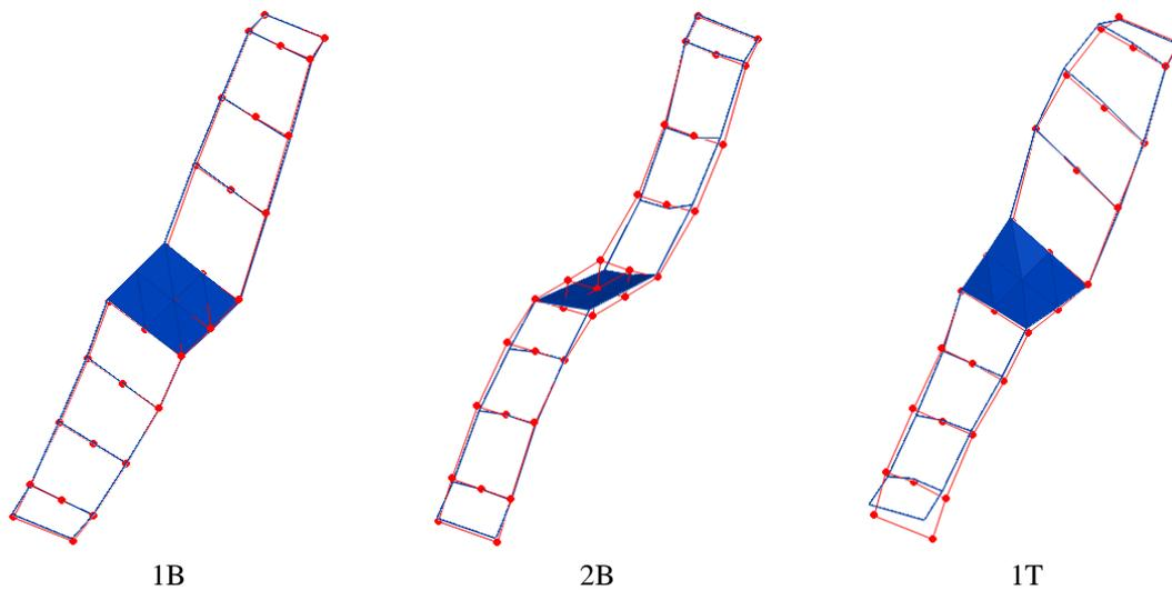
Figure 14. Overlaying of mode shapes obtained experimentally (dotted line) and numerically in the final FE model (solid line)
