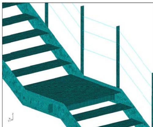
Figure 4. Detail of the FE model of the staircase
