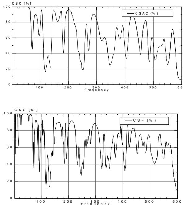
Figure 1. Initial CSAC (top) and CSF (bottom) function for 0-600 Hz.
