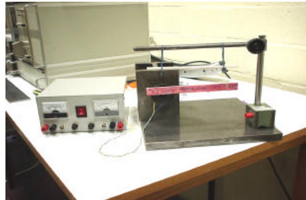
Figure 5: Experimental test set-up with the suspended IPC test beam.
