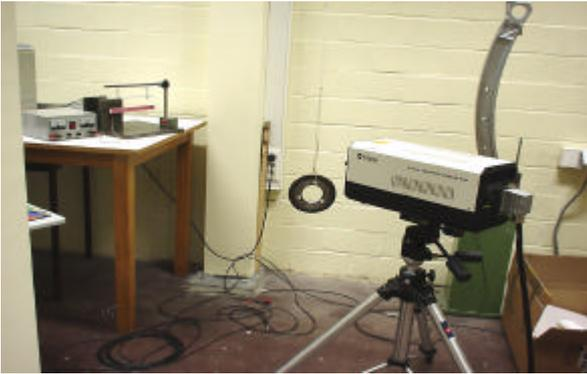
Figure 6: The scan head of the PSV (Polytechnic Scanning Vibrometer)
