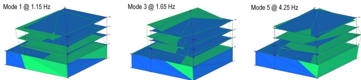
Figure 2. Mode Shapes of P block for OMA- Mode 1, Mode 3 & Mode 5
