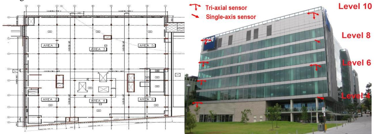
Figure 1. View of P block sensor arrangement and level 1 floor layout.
