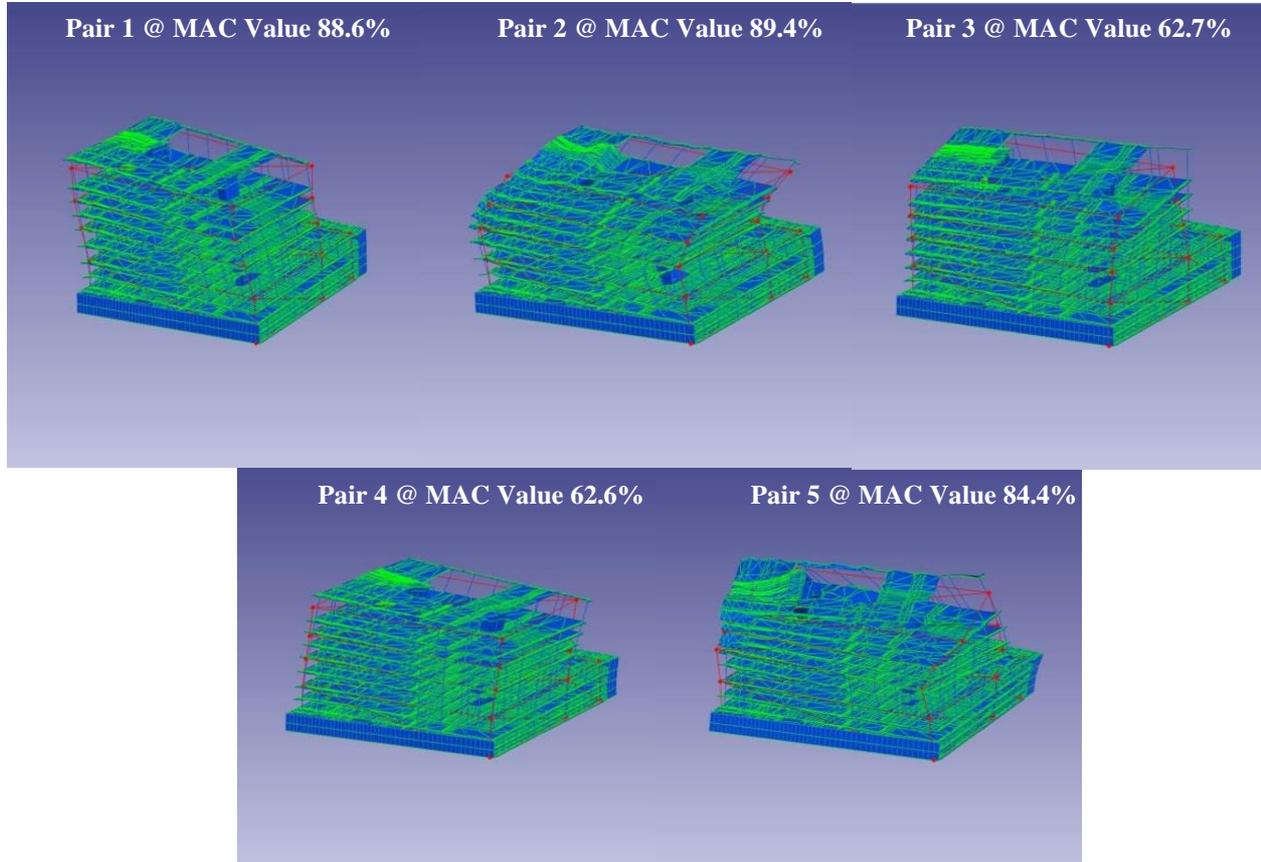
Figure 3. Comparison of FE mode shapes of updated model and OMA mode shapes of P Block
