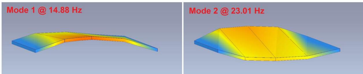
Figure 5. First two mode shapes of the foot bridge
